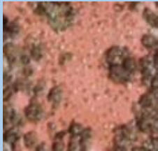
Immersion test (static) in the Seto Inland Sea After 2 months in summer
