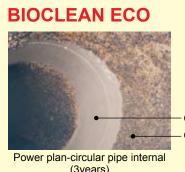
**BIOCLEAN ECO prevents adhesion of marine** growths and shellfish by degenerating lower surface tension silicone synthetic resin by specific surface conditioner that resembles epidermal of dolphin in creating smooth surface. The product has been highly appraised as eco friendly anti-fouling system in many power plants globally.
