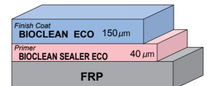
\*1 : Dry film thickness ( D.F.T. ) should be specified according to owner's requirements.
