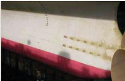
Both trials and In service performance of the silicone coatings demonstrate their ability to keep the surface clean and smooth.
