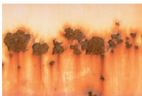
■ Area of heavy rusting and / or defected coatings
