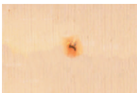
■ Area of light rusting and / or defected coatings
