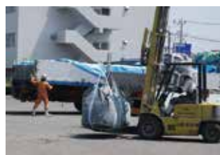
Delivering raw materials by flexible container bags (Kyushu)
