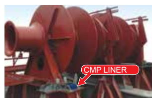
Epoxy resin for chocking CMP LINER
