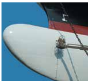
Silicone foul release coating CMP BIOCLEAR
