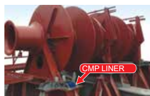
Epoxy resin for chocking CMP LINER
