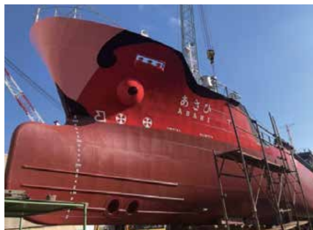
Electric propulsion tanker 'Asahi' under construction (after application of SEA PREMIER 3000 PLUS).
