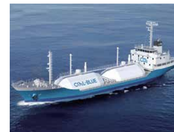
Liquefied CO 2 carrier
