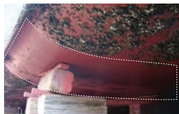
Test coating results of high-performance antifoulings (the dotted line indicates areas with high-performance coating, while the remaining areas have a general-purpose coating)
