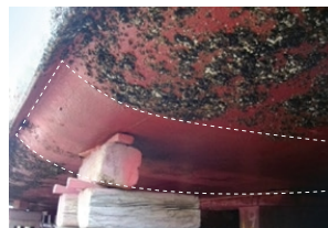
Test coating results of high-performance antifouling (the dotted line indicates areas with high-performance coating, while the remaining areas have a general-purpose coating)
